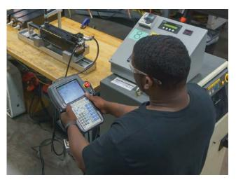
Final system test ensures the feedback device is properly aligned with the ServoWeld motor poles.
